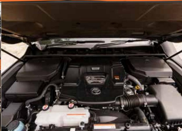
3.3L V6 TWIN TURBO DIESEL ENGINE
